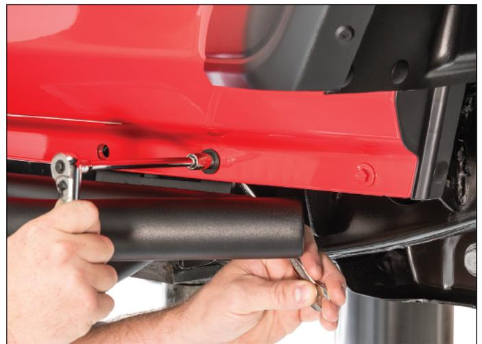
Starting toward the front of the vehicle, position the mounting tabs of the steps BEHIND the pinch seam and align the holes with the factory pinch seam holes. Install the M6 hex head bolts through the pinch seam and the mounting bracket with 6mm flat washers on both sides and secure with a 10mm nylock nut using a 10mm wrench and 10mm socket. Do **not** fully tighten at this time. Repeat for the three remaining holes.
