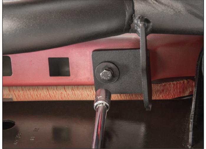
Locate the two vertical threaded holes behind the pinch seam where the brackets were just installed AND the two remaining body mount tabs. Using a 13mm socket and extension, loosely insert the M8 bolt (C), lock washer (J) and flat washer (I) to attach the side step to the body mount. There are four on each side of the vehicle. Tighten enough to hold the step but loose enough that the step can still be maneuvered while attached.
