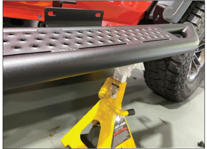
Put on safety glasses. Locate the 4 holes along the factory pinch seam of your vehicle. We will use these to help line up the steps prior to installation. Using a helper or jack stands roughly align side steps to the correct area. Note: On either side, the Quadratec logo will be located on the steps, toward the front of the vehicle.
