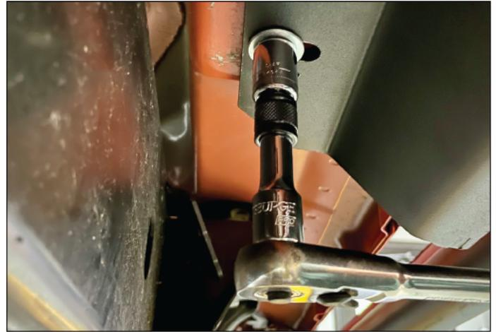
Using the M10 hex bolt (C) with a flat washer (H) on each side and a 17mm Nylock nut (F) attach the bracket to the tab on the steps. Tighten all bolts beginning with the eight pinch seam bolts. Tighten the two bolts that mount from the bracket to the step, and then tighten the four body mount bolts fully. Make sure all bolts are fully secure and torqued to the specifications listed below before using step.
